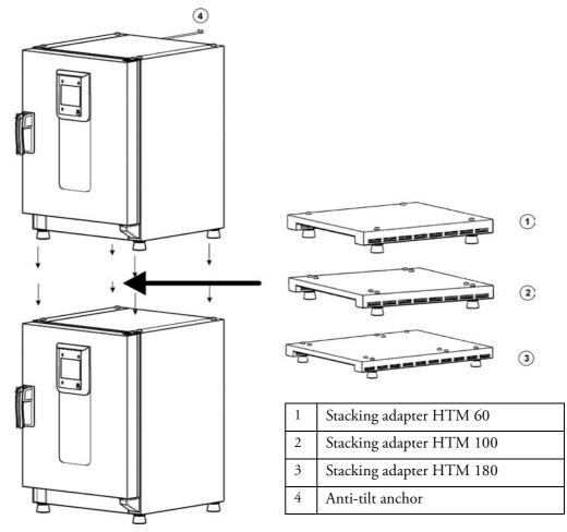
Stack as follows when using a stacking adapter (numbers denote oven volumes in liters):
