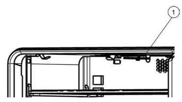
Figure 4-14 Sensor Mounting Location - OMH Series - Table-top ovens
