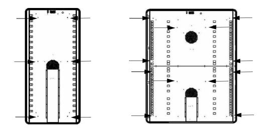
Figure 5-10 Removing the rear air baffle OMH 400/750
