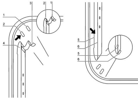
Figure 5-4 Support Rail Installation
