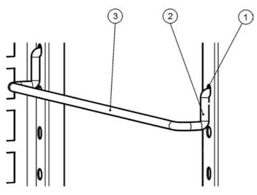
Figure 5-11 Shelf Support Bracket Installation
