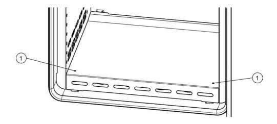
The following section describes the installation and removal of the lateral air baffles.
