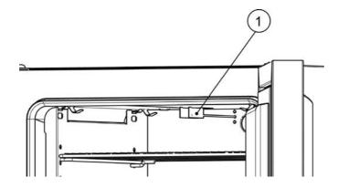
Figure 4-13 Sensor Mounting Location - OGH Series - Table-top ovens
