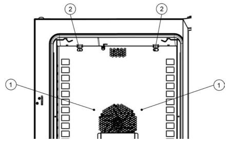
Figure 5-5 Installing the Rear Air Baffle
