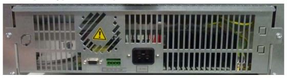
Figure 4-16 Signal Interfaces and Power Socket
