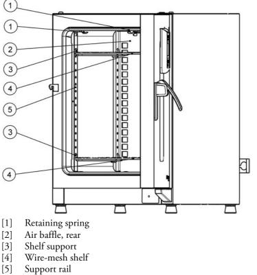
Figure 5-3 OMH and OMH-S Series - Installing the Shelving
