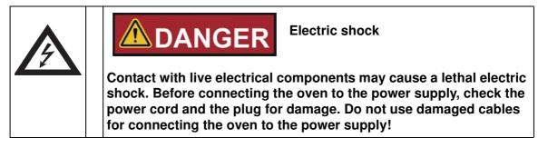
The oven has a class I, protection-earthed enclosure. To minimize the risk of electrical shock, use the AC power cord supplied to connect the oven to a correctly installed and protection-earthed power supply source, with the following features in place for each oven:
